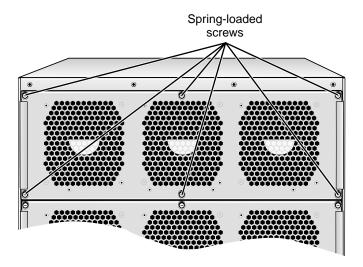
**2** Grasp the two handles on the fan tray, and firmly pull the fan tray toward you (Figure 3).
